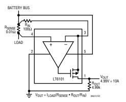
Figure 1. Simple LTC6101 High Side Current Sense Amplifier
